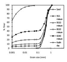
Fig. 1 Gradation curves of different mixtures
