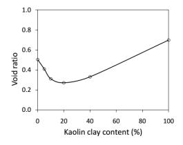
Fig. 2 Curve showing the effect of kaolin clay on void ratio
