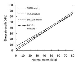
Fig 3 Failure envelopes of sand-kaolin clay mixtures as previously presented by authors in [15]
